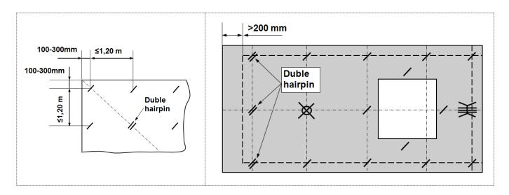
The maximum distance between hairpins must not exceed 1.2 m. For large adhesion forces to the formwork, such as textured finishes, the maximum distance between hairpins must not exceed 0.9 m. The positioning grid for the hairpins must not exceed or fall below the ratio 3:4 or respectively 4:3.
